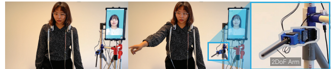
Figure 7: The system tracks the user’s arm direction and visualizes hand pointing direction (Left). The pointing is rendered through the 2 DoF pointing arm attached to the mobile robot (Right).
