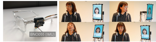
Figure 13: Wearable glasses device with an IMU sensor for tracking head orientation (Left). Demonstration of the articulated display following the user’s right, left, up, and down head movements (Right).
